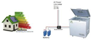
Battery Power with AC automatic Switch
